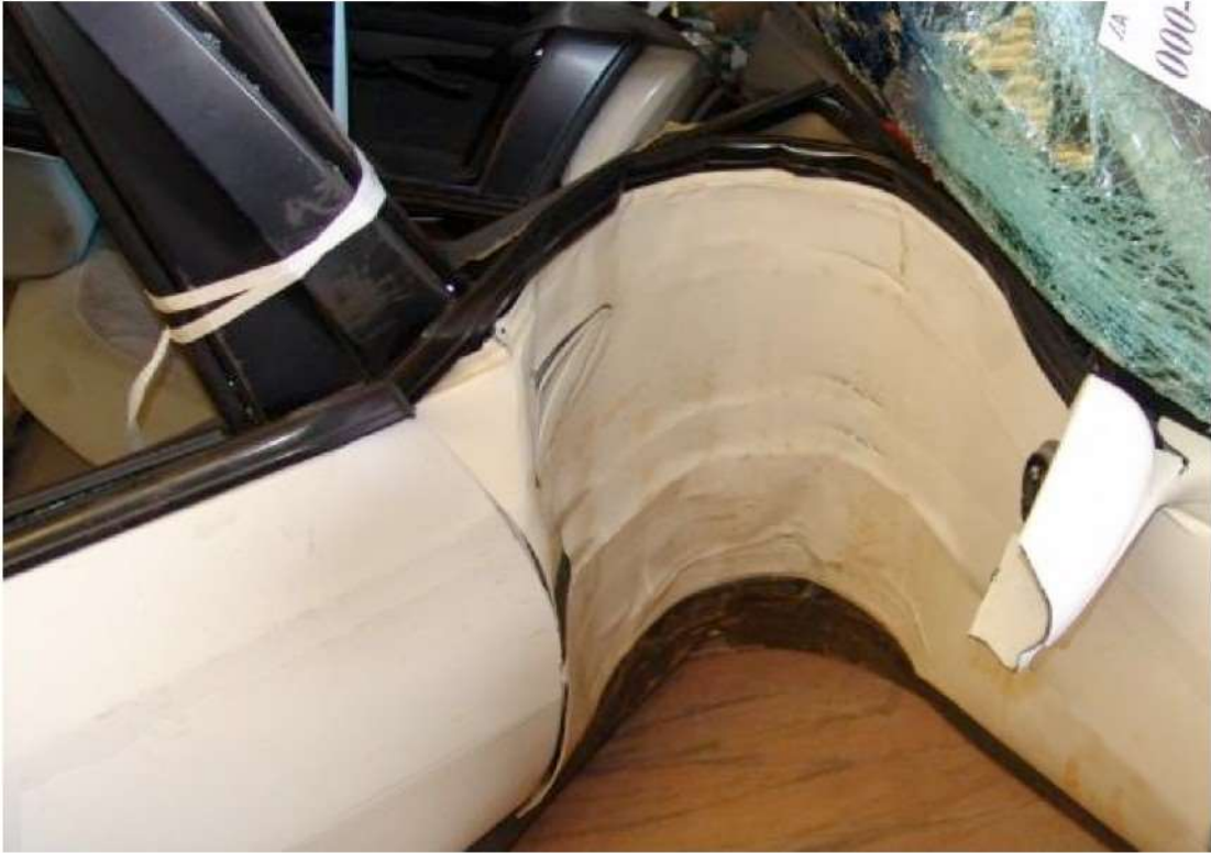
Photograph 0009: Deformed right front door due to contact with tree.
