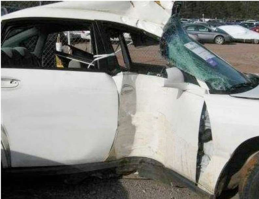
Photograph 0008: Deformation evident at right front door due to contact with tree.
