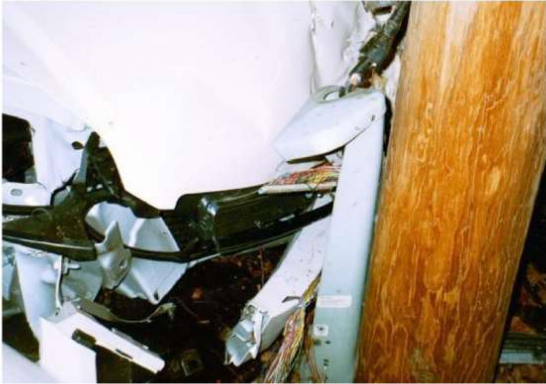
Photograph 0007: Front bumper structure deformed by contact with utility pole (police photo).
