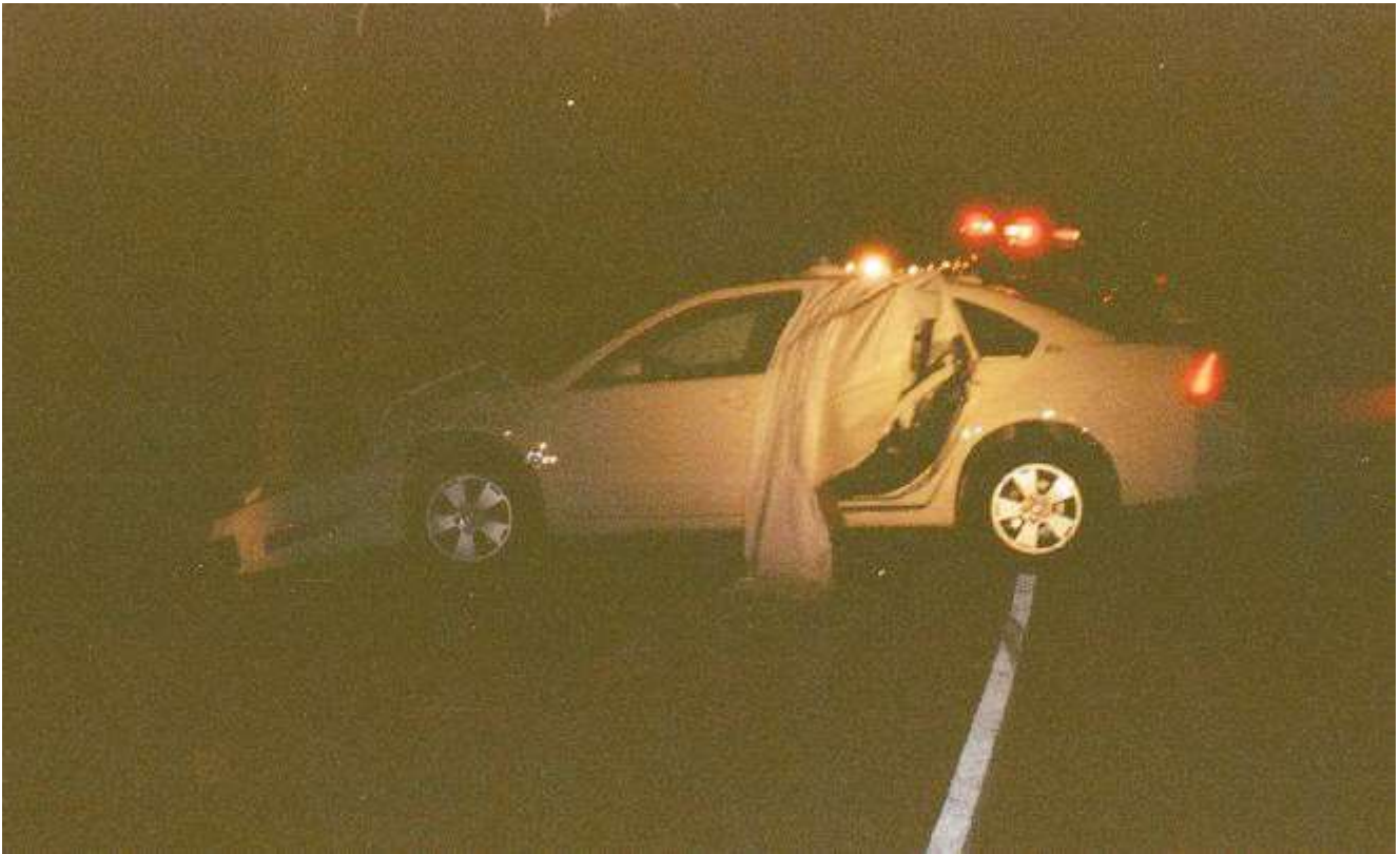
Photograph 0001: Vehicle at final rest. Rear tires remain on paved surface. Front of vehicle at rest against utility pole and right side of vehicle in contact with a tree (police photo).
